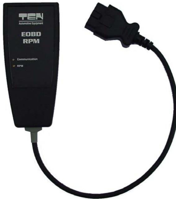
The TEN EOBD RPM is a digital EOBD engine speed sensor which can be used on all existing TEN multigas analysers and smokemeters. The EOBD RPM is connected on the EOBD connector of the examined vehicle and through a connection cable mounted on the multigas analyser/smokemeter.
